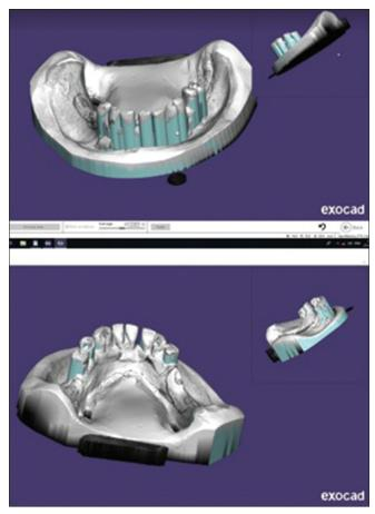
**Figure 2:** Virtual determination of path of insertion and virtual block out of undesirable undercuts.
