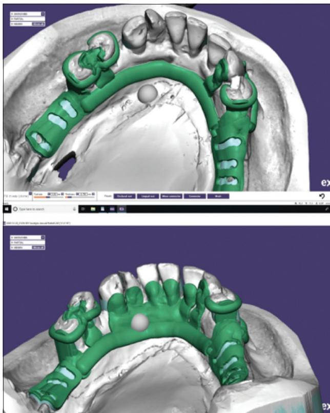
**Figure 3:** Designing the Linguoplate major connector and rests.
