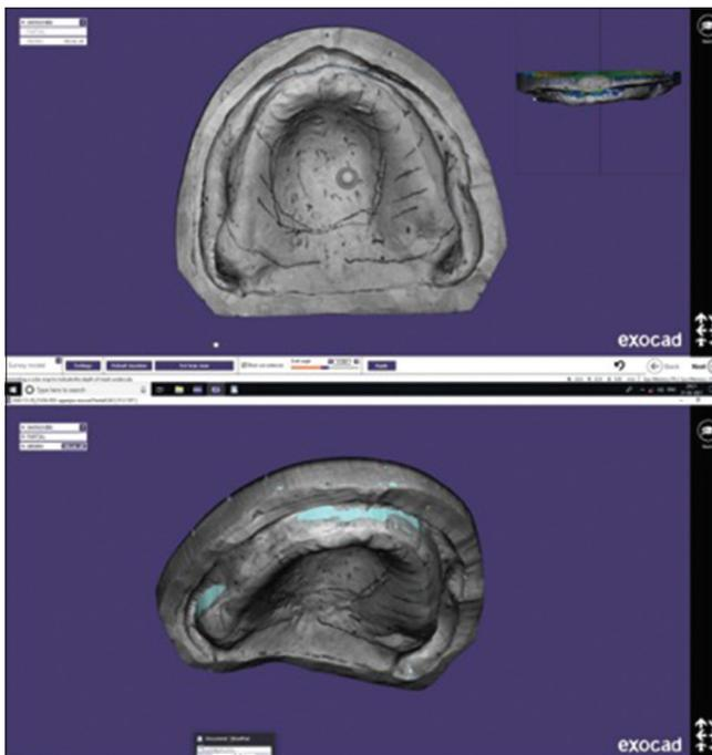
Figure 6: Virtual determination of path of insertion, digital surveying, and block out.
